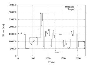
Figure 2. Bitrate obtained with the proposed algorithm and available bitrate, sport video.
