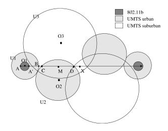
Figure 4. Path of the user and disposition of 802.11b and UMTS cells.
