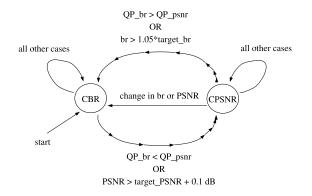
Figure 1. State diagram of the proposed algorithm.
